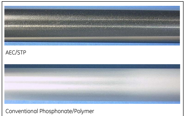
Calcium carbonate deposition studies under heat transfer conditions at 135°F (57°C), pH 8.6, 600 ppm Ca Hardness and LSI 2.5 for 6 Days.
